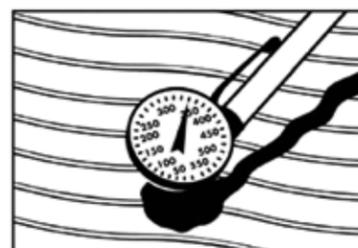
**7** Use a calibrated thermometer to check setpoint
